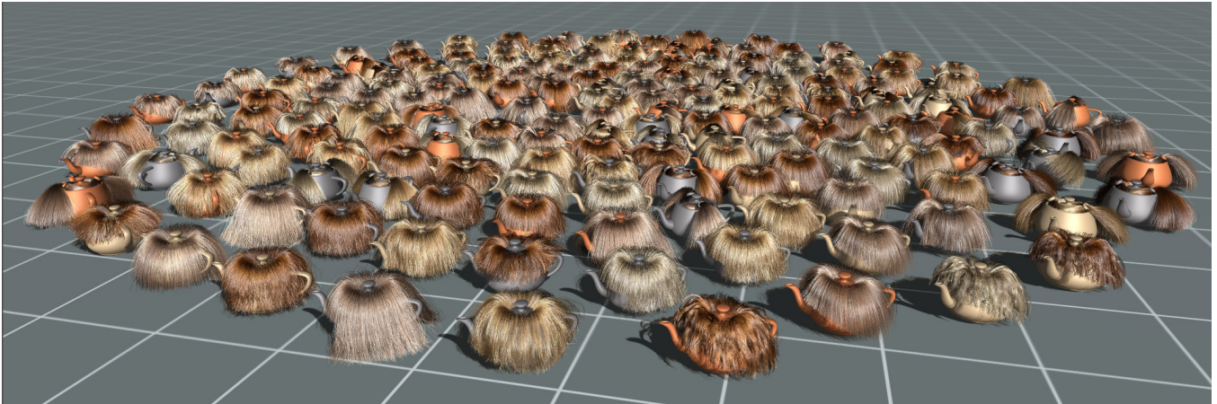
Figure 9: 200 Utah teapot models with unique hair models. Each hair model includes 50 thousand hair strands with a different set of styling parameters. The hair meshes are simulated to generate the hair animations. All hair in this scene is rasterized in 1.8 ms in total with 8x MSAA. Our 5 textures for 200 separate hair mesh models in this scene fit in 3.2 MB (17 KB per teapot on average).
