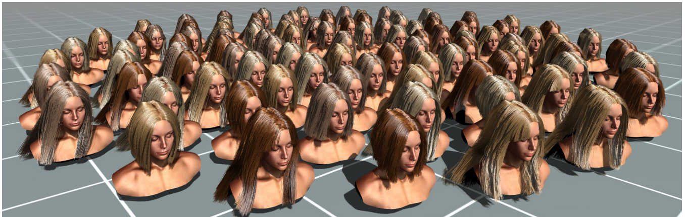
Figure 1: A scene with 100 characters, each with a unique hair model comprising of 100 thousand strands, rasterized in only 2 ms on an NVIDIA GTX 4090 GPU (with 8× MSAA) using our real-time hair rendering method with hair meshes and our level-of-detail techniques. All 100 hair mesh models in this scene fit in 1.7 MB (between 13 KB and 21 KB per model).
