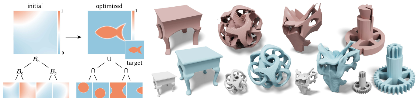
Fig. 1. We develop a unified boolean operator \mathcal{B}_c that is differentiable with respect to the type of boolean operations. In the context of inverse CSG, starting with randomly initialize primitives and boolean operations (left tree), our method enables continuous optimization on both the primitives and the boolean operations in order to fit the target shape (middle tree). Performing inverse CSG fitting to the ground truth shape (grey) with our method leads to significant quality improvement (blue) over the traditional boolean operations with the min and max operators (red).
