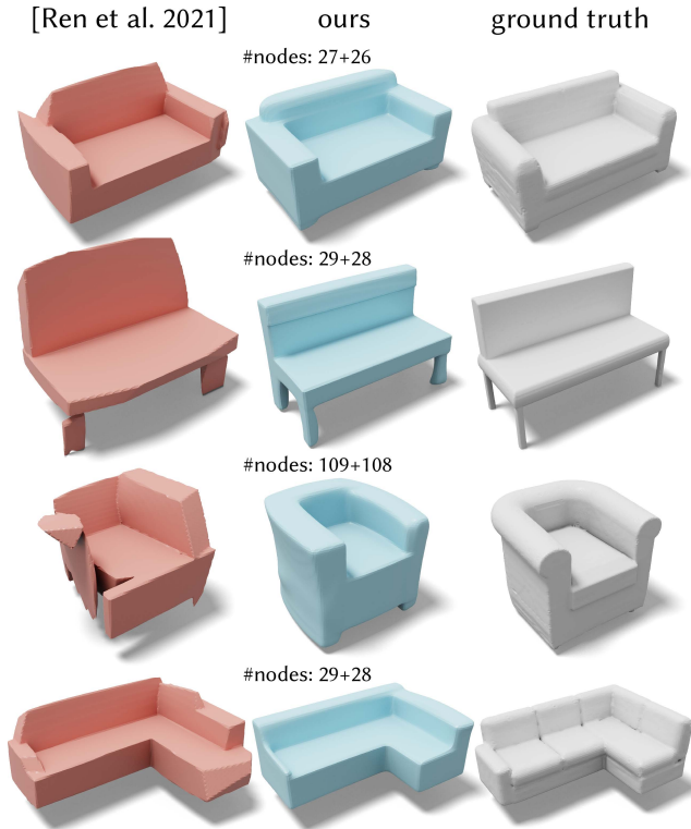
Fig. 13. By simply replacing the CSG tree structure in [Ren et al. 2021] with our method, our approach can obtain qualitative improvement in fitting the ground truth shape over their approach. We also report the number of nodes ( \#primitives + \#boolean ) after pruning for our method. Note that the raw output of [Ren et al. 2021] requires around 15K boolean operations with many redundant ones. Thus, we do not report their number because a pruning method for them would be required for a fair comparison on the compactness of the tree.
