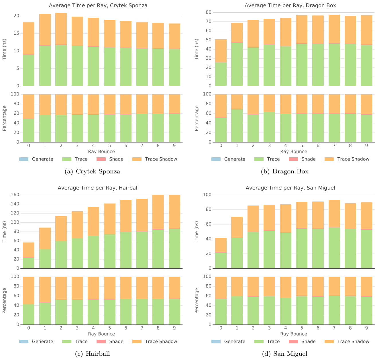
Fig. 6 Classification of time per kernel normalized by the number of rays. Each scene rendered with maximum of 9 ray bounces. Note: contributions from the Generate and Shade kernels are negligible compared to others. Shadow Trace is somewhat less expensive than Non-Shadow Trace due to algorithm optimizations.
