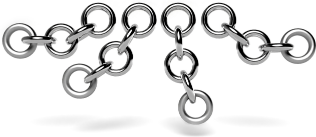
Fig. 22. 5 rigid bodies, each with 6 DoF, forming a chain through collisions, simulated using our VBD formulation for rigid body dynamics.
